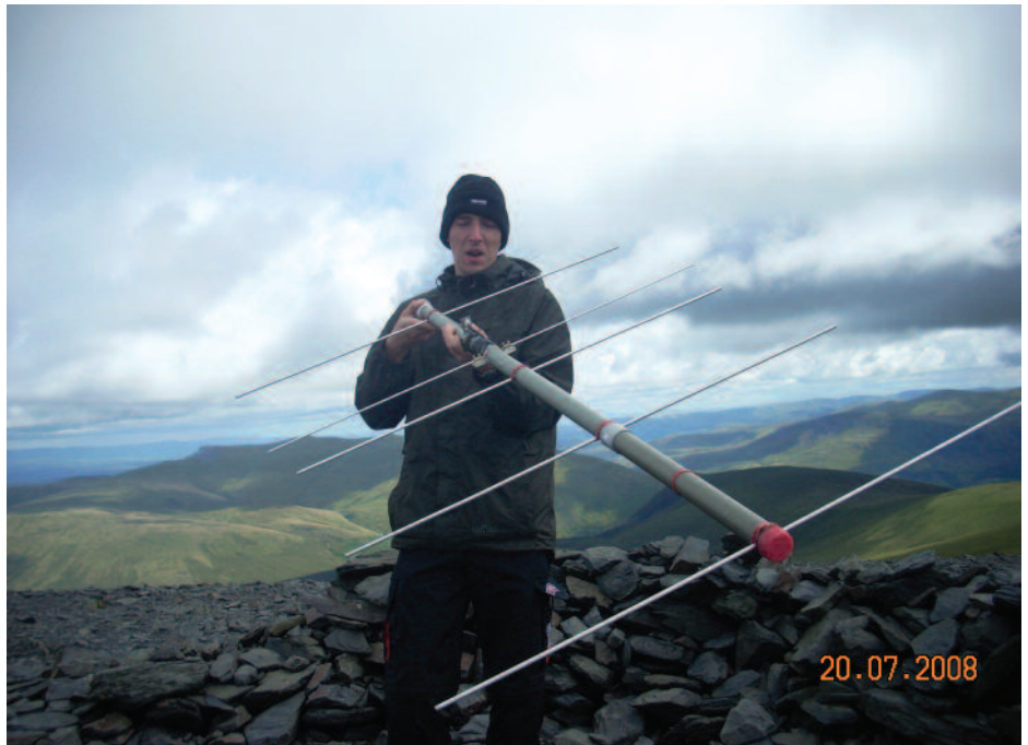
John, MOUKD holds the home made 5-el 144MHz beam.
